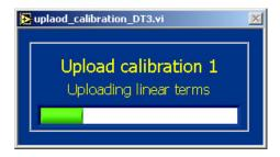
After uploading the calibration do not forget to turn off the unit and REMOVE the jumper from the two pins on the back of the unit. Only DT-100C-IS model with 6 calibrations needs this jumper ALL TIME IN PLACE when working with *DT/JT Commander* software, to be able to send data to RS232.
