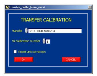
The "Reset unit correction" option should be used very carefully, because it sets the unit correction slopes to one and the unit correction intercepts to zero and therefore affects all calibrations!
