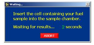
Pressing F2 or the "Measure" button shows a window that prompts you to insert the cell containing your sample into the sample chamber of the instrument. If done, the sample is analyzed, the window is closed automatically and the results are shown in the main window. Beside the calculated concentrations also the absorbances of the different wavelengths are shown.
